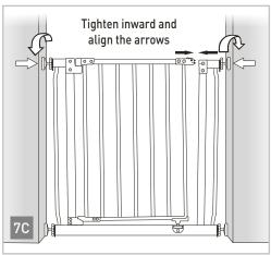
8. Tighten the Tension Knobs until the two Arrows, located on the Upper Locking Set and on the Right Upper Corner, align horizontally (8A).
