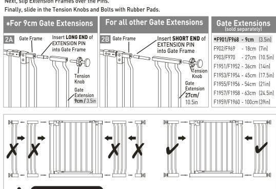
1 on each side of gate. Do NOT install 2 Gate Extensions on the same side of gate.
