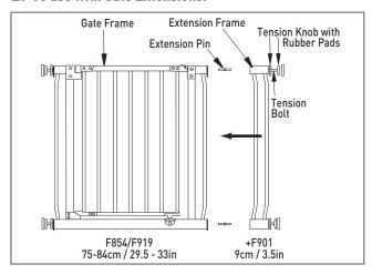
Insert Extension Pins into the holes on the outside of the Gate Frame (2A / 2B). Next, slip Extension Frames over the Pins.
