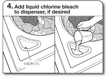
Do not overfill, dilute, or use more than 1 cup (250 mL). Do not use color-safe bleach or Oxi products in the same cycle with liquid chlorine bleach.
