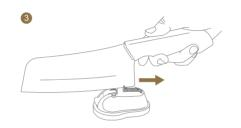
Place the knife in the gap and pull the knife backward. Press the knife slightly strong and you will have more sharper knifes.
