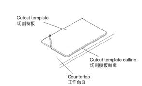
Trace the outline of the cutout template on the countertop with a pencil at the desired installation location. 用鉛筆在廚房工作台面上您希望 安裝水槽的位置畫下切割模板的輪廓。
