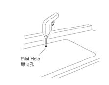
Cut along the outline to cut out the opening in the countertop 沿著劃出的輪廓線切出 水槽安裝孔
