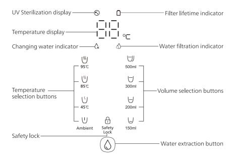
There could be a temperature deviation of  $\pm 3\,\mathrm{C}$  and a volume deviation of  $\pm 10\%$ , the actual temperature and volume depends on usage environment and local tap water quality.
