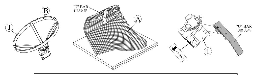
CAUTION: Failure to place "U" metal plates (F) under the rocker plates (I) and above the "U" bar exactly as shown in the diagram will cause the bolt heads and nuts to damage the structure of the rocker plates and the "U" bar. Damage due to over tightening of bolts or improper assembly could cause injury and may void your warranty.
