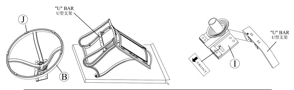
CAUTION: Failure to place "U" metal plates (F) under the rocker plates (I) and above the "U" bar exactly as shown in the diagram will cause the bolt heads and nuts to damage the structure of the rocker plates and the "U" bar. Damage due to over tightening of bolts or improper assembly could cause injury and may void your warranty.
