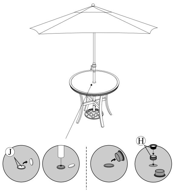
If using a small umbrella with a pole less than 1.4 in / 3.8cm, replace part J with part H. 如使用雨傘的直徑是少於1.4英寸/3,8公分,請使用零件H取代J.
