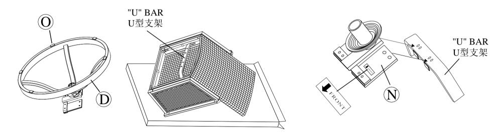
CAUTION: Failure to place "U" metal plates (H) under the rocker plates (N) and above the "U" bar exactly as shown in the diagram will cause the bolt heads and nuts to damage the structure of the rocker plates and the "U" bar. Damage due to over tightening of bolts or improper assembly could cause injury and may void your warranty.
