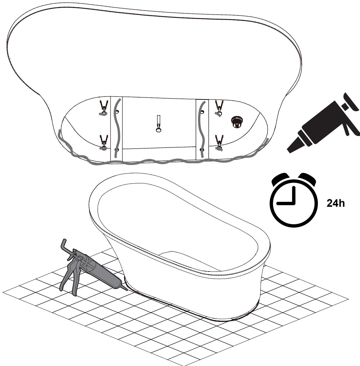
**BEFORE FIXING YOUR TUB TO THE FLOOR, MAKE SURE YOU HAVE INSTALLED YOUR FAUCET (if applicable) AND THAT YOU HAVE CHECKED FOR LEAKS.**
