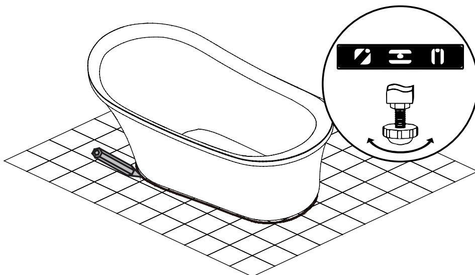
1. Place the bathtub in the desired position on the floor and level it using the adjustable feet.
