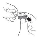
Attach the automatic milk frother to the milk frother lid. When the two parts lock into place, you hear a click.
