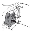
10 Slide the brew group back into the machine along the guiding rails on the sides until it clicks into position.
