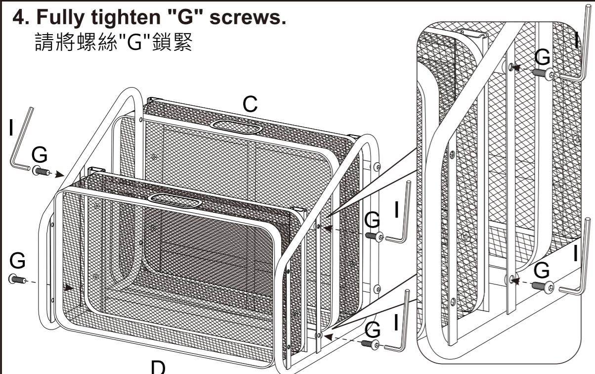
**5. Fully tighten "G" screws.**
